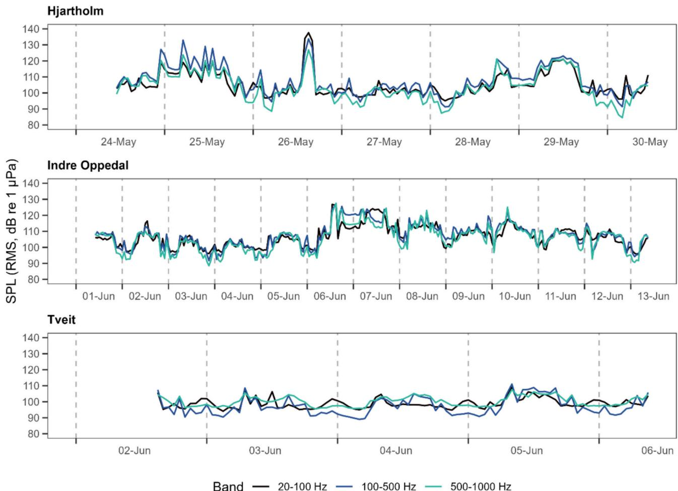
**Fig. 6.** Temporal patterns in the root-mean-square sound pressure level ( $SPL_{RMS}$ ) at 3 sea-cage salmon farms in Sognefjord, Norway. Sound levels were calculated at hourly intervals over 3 frequency bands. Delousing wellboats visited Hjartholm (24–26 May and 28–29 May) and Indre Oppedal (6–12 June). Tveit was only visited by workboats conducting routine activities.
