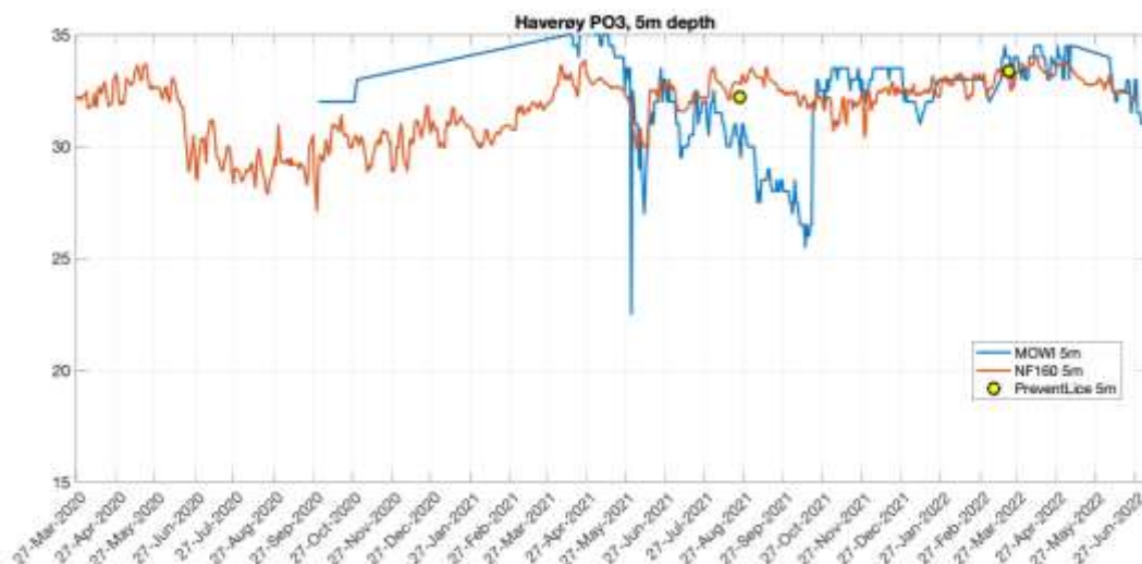
Figure 18: Salinity at 5m depth at Haverøy on the western side of Sotra. Observations (blue) and model results from NorFjords 160 (red). Yellow dots indicate the times when there was a project sampling measurement at this location.
