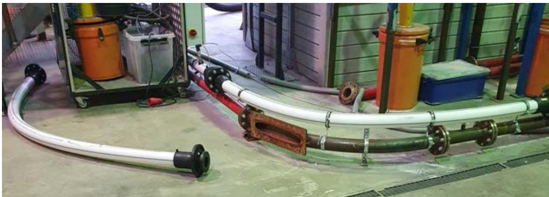
Figure 13: Two bend segments with flanges fabricated by Bilfinger.
