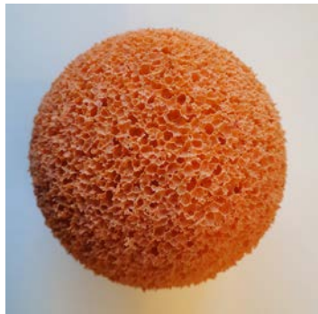
Figure 7: A cleaning sponge kindly provided by AKVA group for cleaning of feeding pipes.
