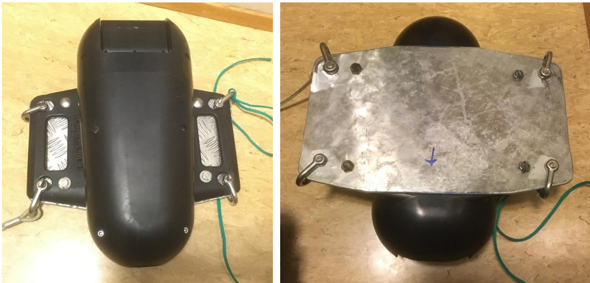
Figure A2 – the JT Electric Trawl Camera (Left), with a reinforcing base-plate fitted by the Vikingbank's engineers during the cruise (right).
