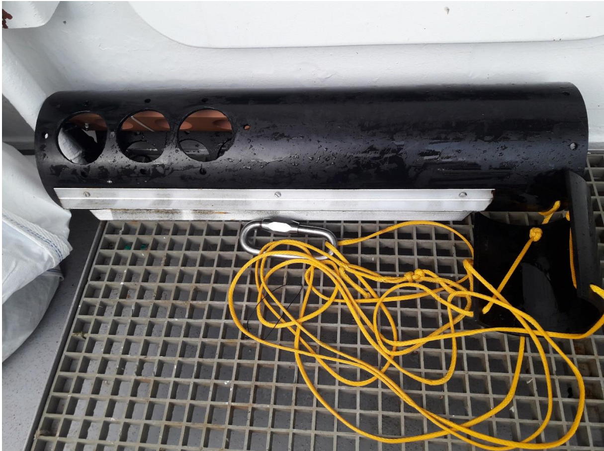
Figure A3 – the “Flying Camera” housing with tether line (Dyneema) and kite [Source: J.Saltskår].
