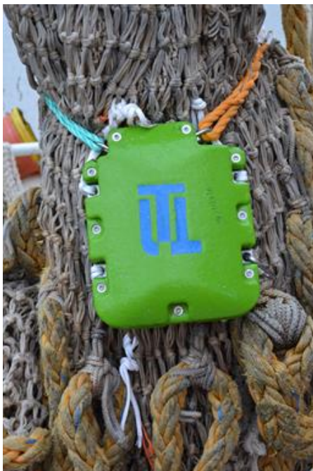
Figure 13: FossTech’s prototype Catch Limitation Release (CLR). Left: CLR unit fitted to codend. Right: restrictor line and fastenings.
