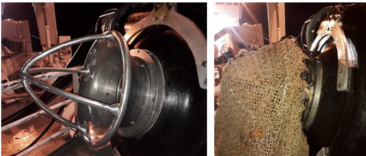
Figure 18 - Left: the pump-head funnel; and Right: pump with pump skirt connected [Source: J. Saltskår].
