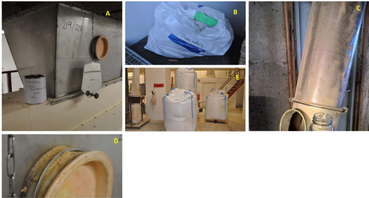
Figure 2.7 - Pictures of the sampling activity at the Skretting facility. A, D = soya protein line; C = wheat gluten line; B, E = plastic bags used for raw material shipment.
