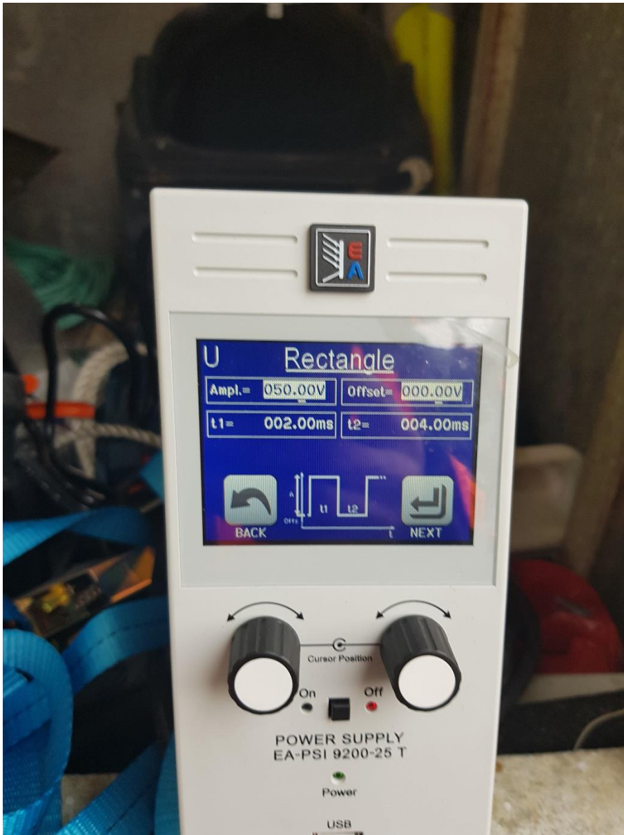
Figur 2 EA Elektro-Automatik Bench Power Supply, 1.5kW, 1 Output, 0 → 200V, 25A
