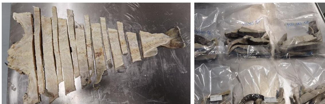
Figure 2: Dec. Lei 25/2005 cross-sectional method. Samples for analysis and desalting.
