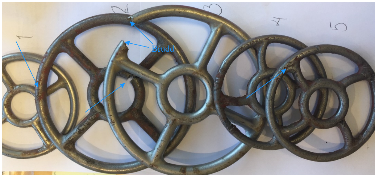
Figur 3. Korroderte stålringer mottatt for evaluering
