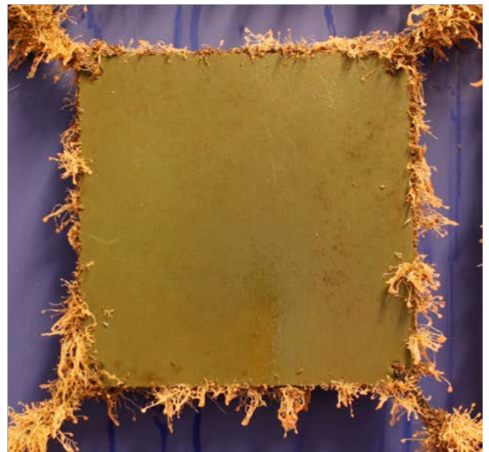
Figure 14: Left: Example of a PVC panel coated with copper shim tape (green/yellow). Where the copper has leached out, the grey PVC base plate can be seen. Right: In comparison, no patchy leaching is visible from the copper-embedded antifouling film.
