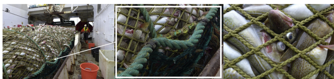
Fig. 1. Codend images taken during the cruise. Picture (a) shows the 2P_Knotted codend normally used by the fleet, picture (b) shows detail of the 2P_Knotted codend, whereas picture (c) shows a detail of the compression of fish against a knotless netting panel.
