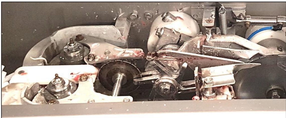
Additional belly cut and new gutting wheel
