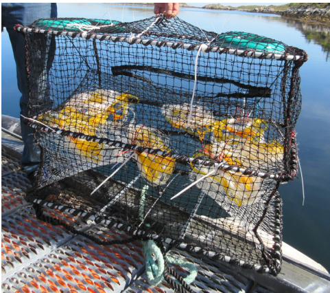
Figure 3. Modified lobster pot with 8 sets of test samples (at Hitra).
