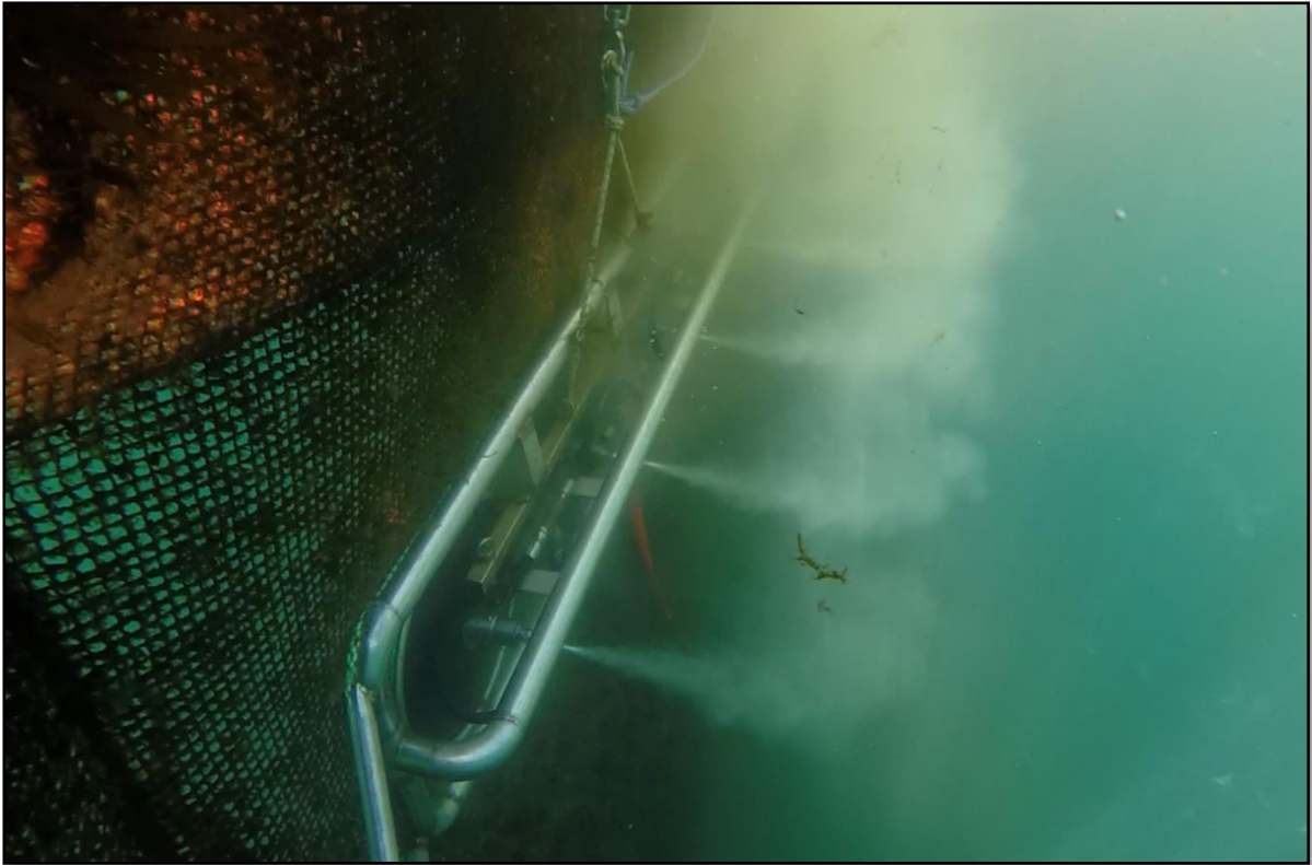
Figure 2.2.3-2. Example of a net cleaning rig from AKVA in action on a net with relatively low levels of fouling. Photograph courtesy of N. Ribeiro, with permission.
