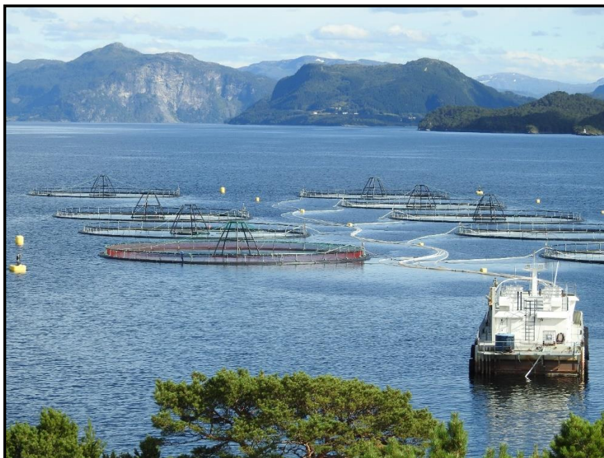
Figure 1.9-1. Feed delivery pipes going from the central feed barge to commercial trout rearing cages. Photo kindly provided by Ola Sveen, Svanøy Havbruk AS.
