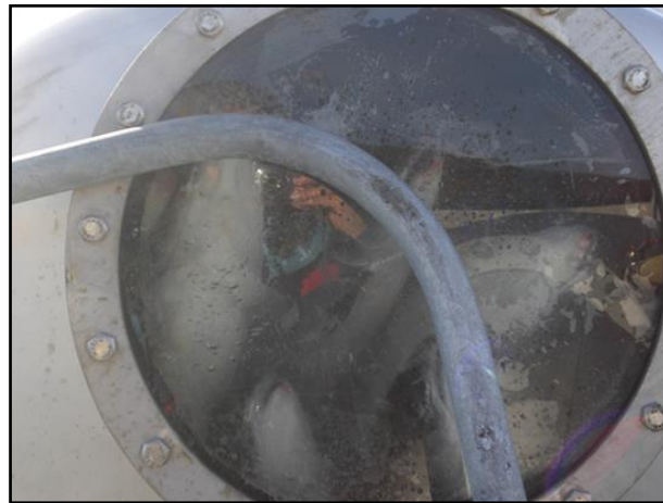
Figure 1.2-4. The behaviour of fish inside the pump. There should not be too much panic activity in the pump and no red water should be seen. Photo: Å. M. Espmark
