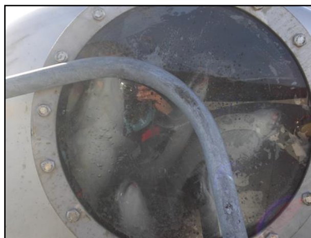
Figure 1.2-4. The behaviour of fish inside the pump. There should not be too much panic activity in the pump and no red water should be seen. Photo: Å. M. Espmark
