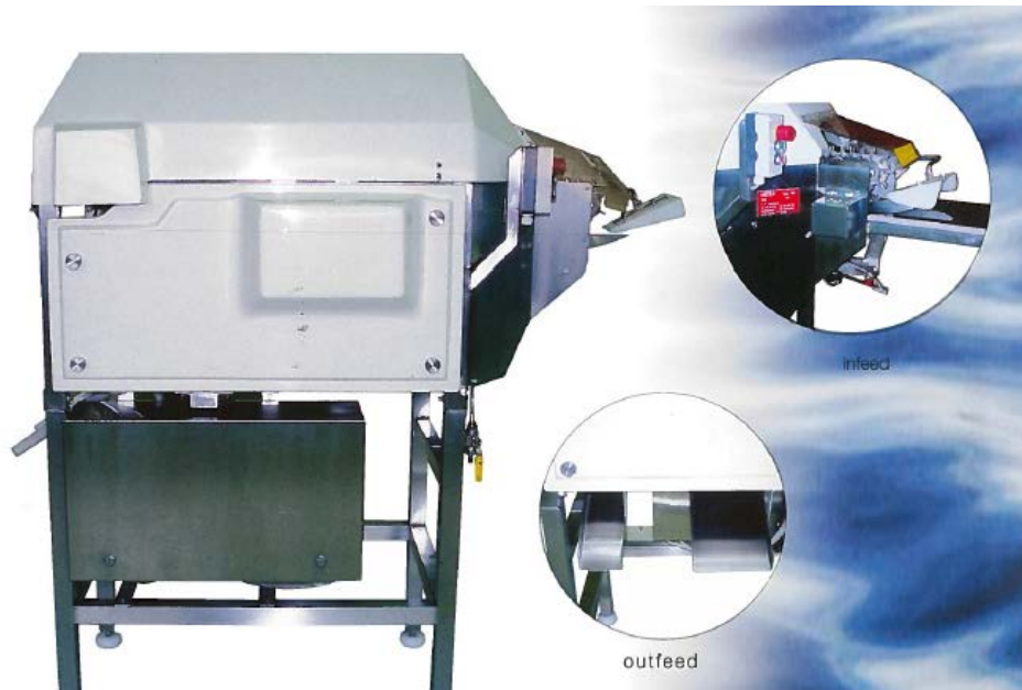
Figur 1. MESA 900 Tongue and Cheek machine (Foto: MESA).
