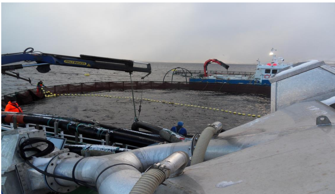
Picture 1. The well-boat used in the first study and fish being pumped from the polar circle into the freshwater well on board.
