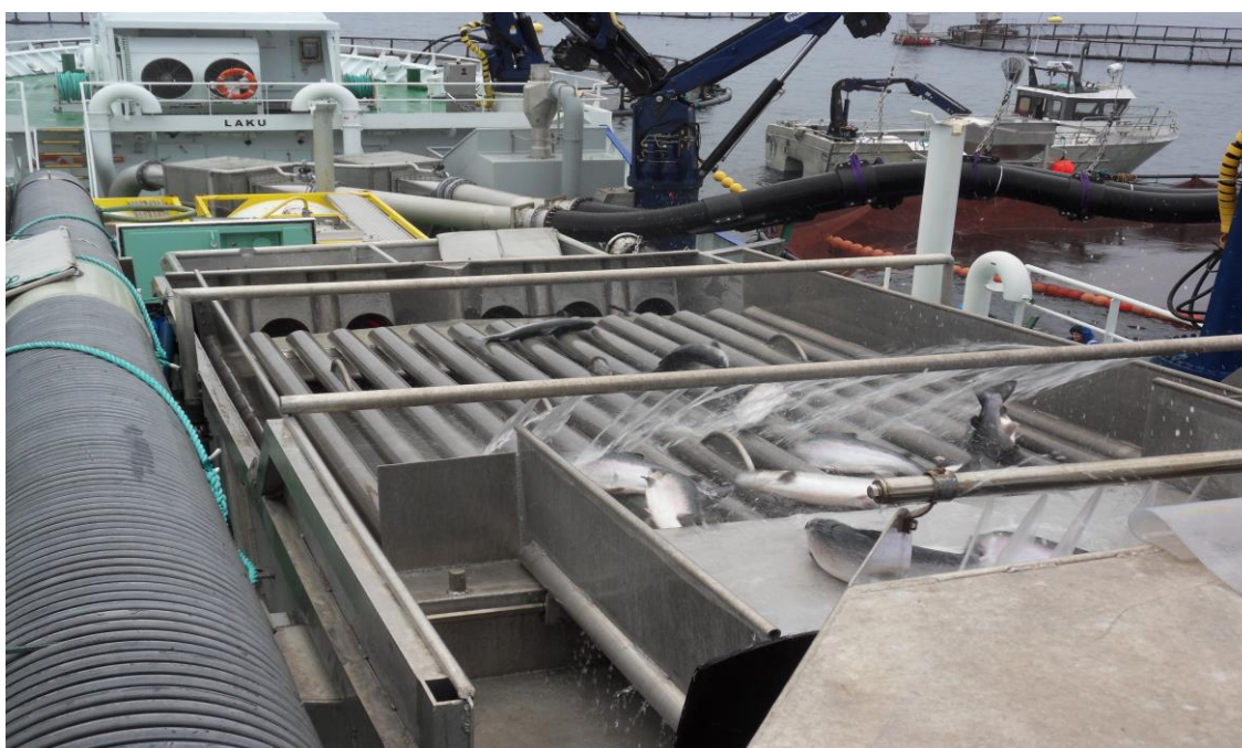
Picture 2. The well-boat used in the second study and fish being pumped from the polar circle into the freshwater well on board.
