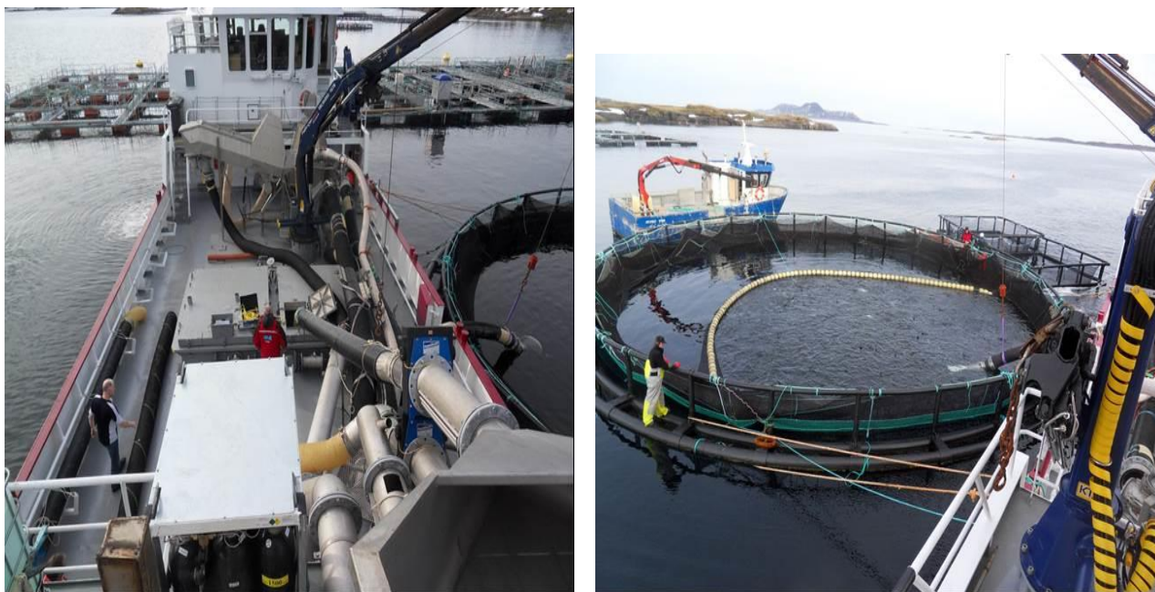
Figure 1. The well-boat used in the study and fish being pumped from the polar circle into the two wells on board.
