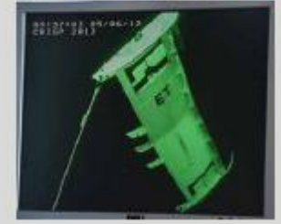
Figure 5.9. 2 m 2 (upper picture) and 9 m 2 (lower picture) trawl doors equipped with hatches, which are used to adjust depth and horizontal spread.
