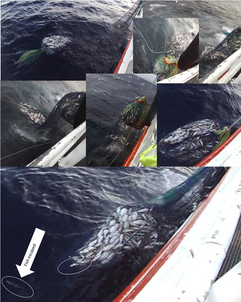
Fig. 3: Collage of photos taken during the "sacking" operation. The photos show how the fish-lift is operated by releasing part of the catch into it while the remaining part of the catch is kept in the square mesh section of the codend at the surface. Several of the photos show that the catch remaining in the square mesh section is surrounded by tensionless square meshes. Further, there is evidence that escapement at the surface does occur.
