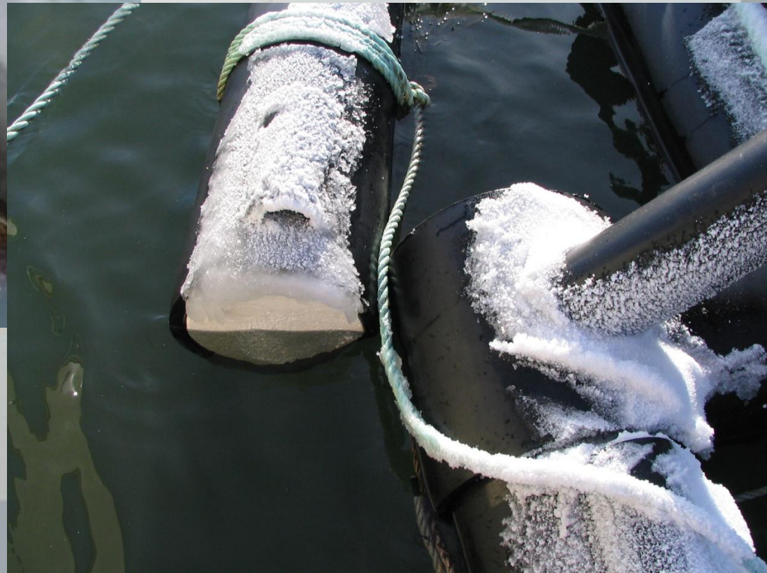
HDPE surface pipe broken
