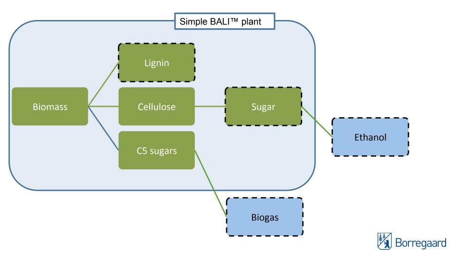
Borregaard biorefinery extended with BALI™ technology Concept: simple Value creation: not very high Site: Where conditions are very good Technology risk: low Simple BALI™ plant Lignin Biomass Cellulose Sugar Ethanol C5 sugars **Biogas**
