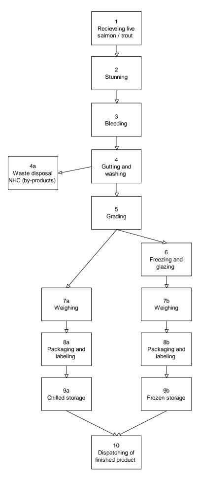
**Figure 1:** Flow diagram of the common steps in the production of dressed salmon and trout from fresh live fish in Norway.
