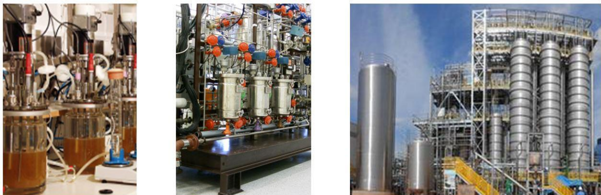
Figure 16. Different fermenting set-ups from lab-scale, pilot-scale and at the industrial scale (left to right). Source: SINTEF Materials and Chemistry and www.amyris.com .
