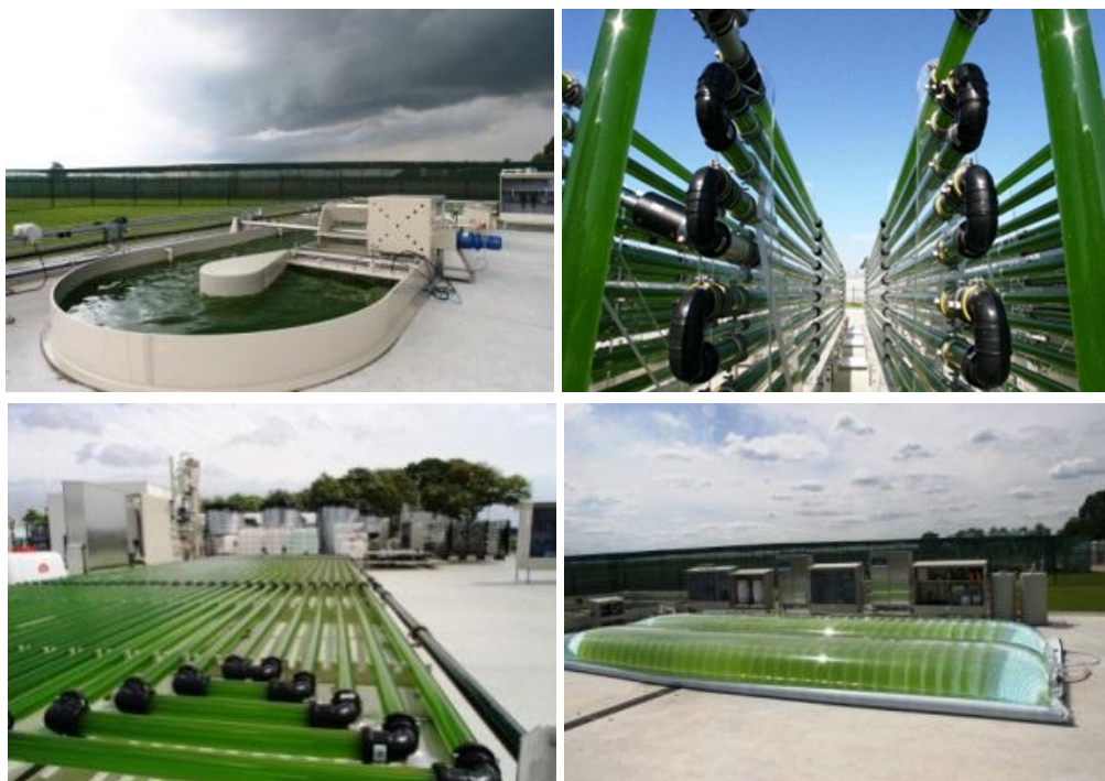
Fig. 11. Pilot production systems of various designs. Top left: Conceptual model of open ponds system. Top right: Closed vertical (3D) tubular PBR. Bottom left: Closed horizontal (2D) tubular PBR. Bottom right: Innovative design of flat panel PBR, enclosed in a water bag for temperature control. Source: AlgaePARC.
