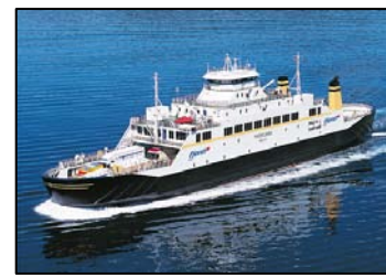
Fjord1 Gassferge (1xC25:33L9AG retrofit)
