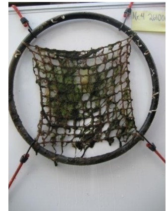
Field test systems for marine growth on fish farm nets (Photo T. Nordtug)
