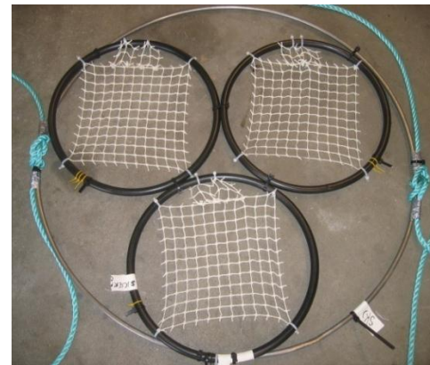
Field test systems for marine growth on fish farm nets (Photo T. Nordtug)
