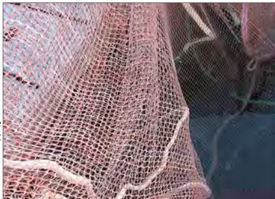
Figure 8. Image taken at termination of the experiment showing no fouling of the cage net. Photo: Nofima
