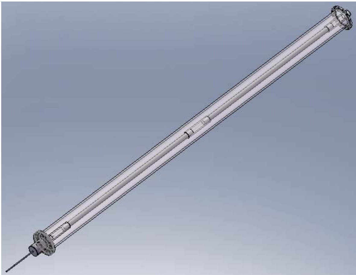
Figure 3.2: Dual pipe design of the test section
