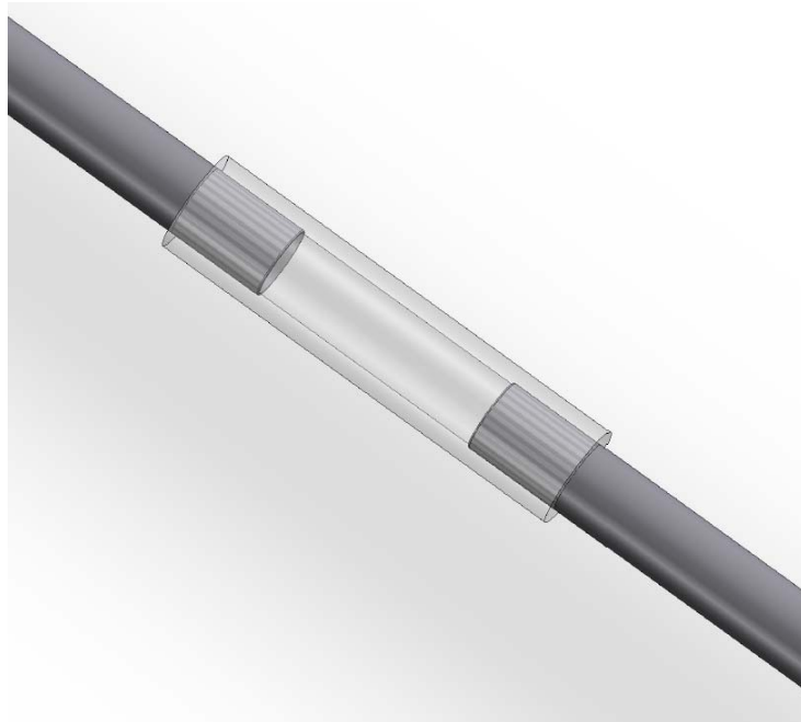
Figure 3.4: Stainless steel and acryl glass pipe combination
