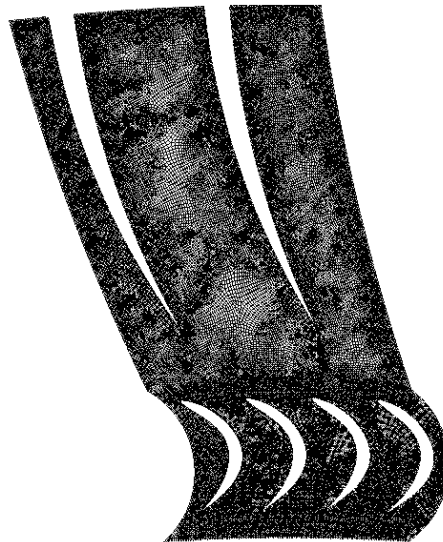
Figure 14. The meshed domain of 1/50 of the full wheel depicting the reference blade shape
