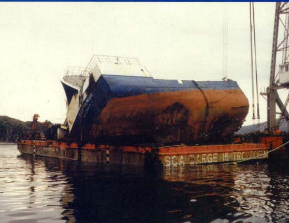
Wreck removal of M/V «Oldersund» with a steelweight of 240 tonn from 10 m. at Rørvik January 1997.
