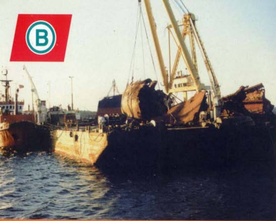
Wreck removal of M/V «Sønnodd» with a steelweight of 550 tonn from 17 m. at Grimstad summer 1999.
