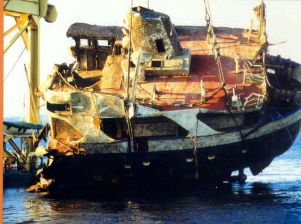
Wreck removal of M/V «Sønnodd» with a steelweight of 550 tonn from 17 m. at Grimstad summer 1999.
