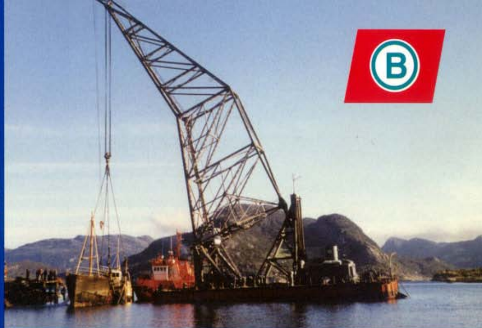
Wreck removal of M/V «Oldersund» with a steelweight of 240 tonn from 10 m. at Rørvik January 1997.
