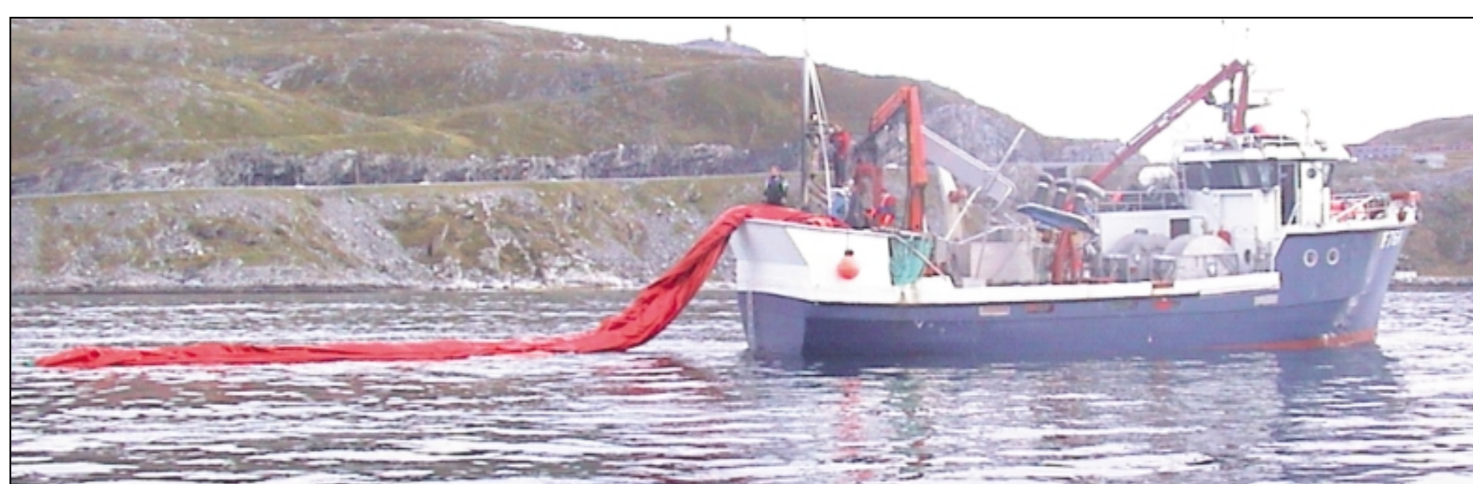
The towing cylinder is set afloat over the stern. It can be towed and kept open by the coastal seiner's life-boat, and is taken on board through the triplex.
