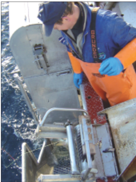
The automated long line hauler from Delitek "delivers" the cod onboard without marks from the gaffer.
