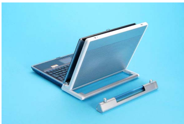
Figure 13 - Fuel cell powered desktop from Fujitsu Laboratories, 2004
