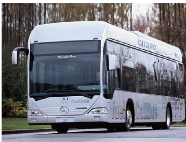
Figure 15 - Fuel cell powered bus in the CUTE - project, developed by DaimlerChrysler
